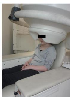
MEG data were collected using an 252 channel CTF scanner, purpose built for adults (see photograph above). The Aston Brain Centre is the first centre in Europe to develop a paediatric-compliant MEG system and facility for the study of brain development in children.
