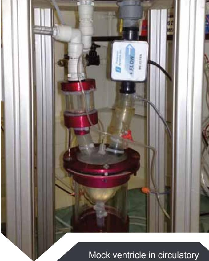
Mock ventricle in circulatory loop: a test facility for cardiac devices.
