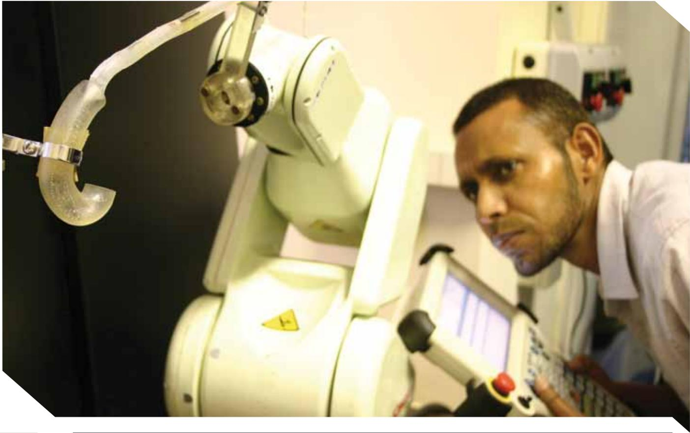
The aim of this research is to develop steerable digits as tool points to aid palpation and navigation in lumen in minimal access surgery. Currently the research is leading to the construction and demonstration of mini-digits with tactile information feedback for clinical processes.
