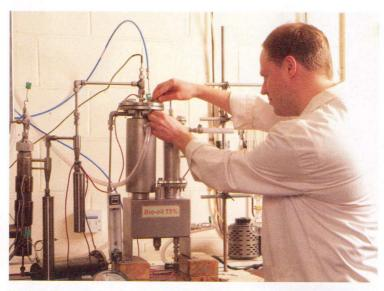
Pyrolysis heats waste in the absence of oxygen, converting it into liquid fuel
